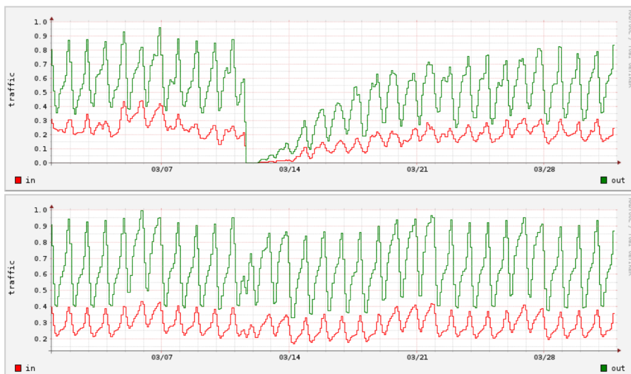
Figure 16: Japanese traffic for the March 2011 earthquake, Miyagi prefecture (top) and nationwide (bottom) [7]
