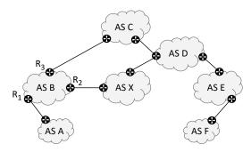
Fig. 1: Where is the lie? Being, A and F stub ASes; B, X and E transit providers; and C and D Tier-1 and Tier-2 ASes, respectively.
